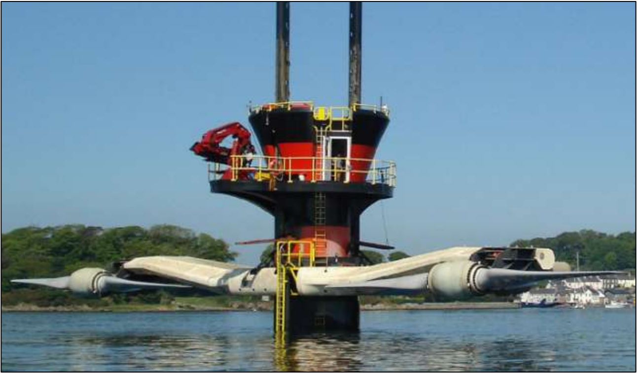
Figure 5:2 - Seagen Device (with Rotors Raised for Maintenance) (Aviation Enterprises, 2012)
