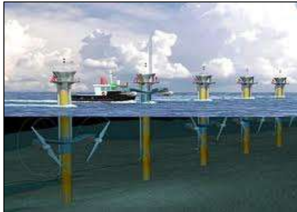
Figure 5:4 - Single Row Configuration (SeaGen 1.2MW)
