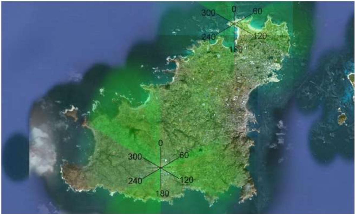
Figure 8 : Satellite image of Guernsey identifying the location of the two anemometers, showing the different sections and their relative exposure to prevailing winds (Lee. O, 2012). Le Chouet is shown to the northeast (top right) and the Airport is shown to the south (bottom middle)
