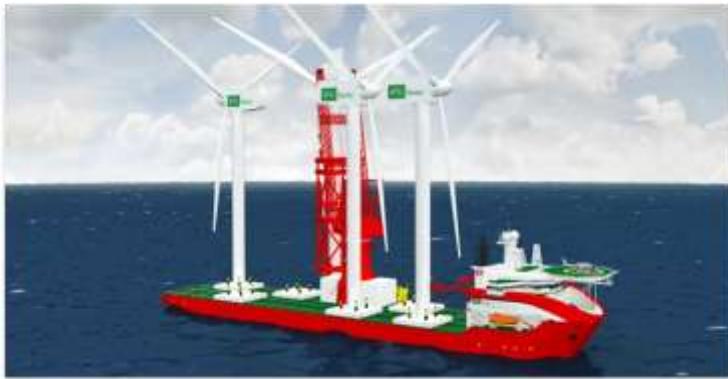
Figure 30 : Vessel displaying fully-assembled installation capability (source W3G Marine)
