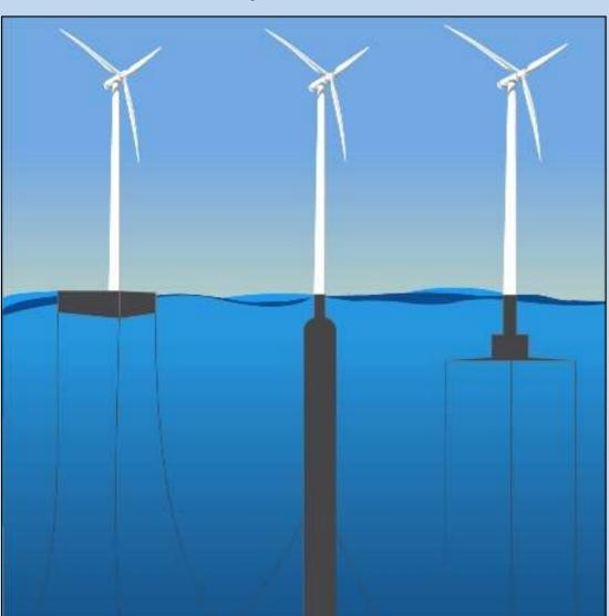
**Buoyancy Stabilized** Barge with catenary mooring lines
