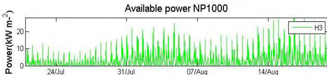
Figure 8.1.3.9: Extractable power output from NP1000 turbine assuming 100% power extraction, independent of cut-in speeds for Site H3 over one month.
