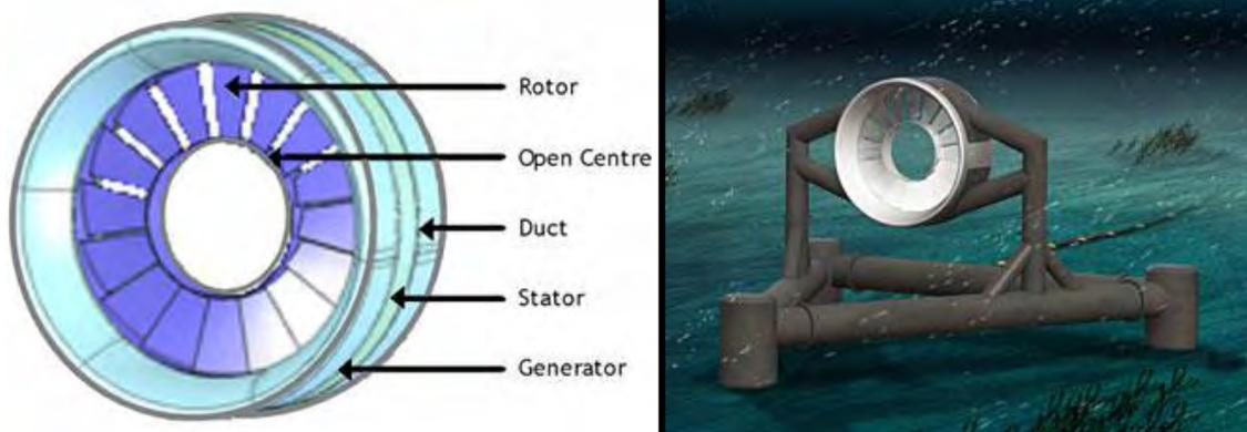
Figure 6.1.5.1: OCT turbine component diagram (left) simulation of turbine mounted on gravity base (right)(Open Hydro Ltd, 2012)
