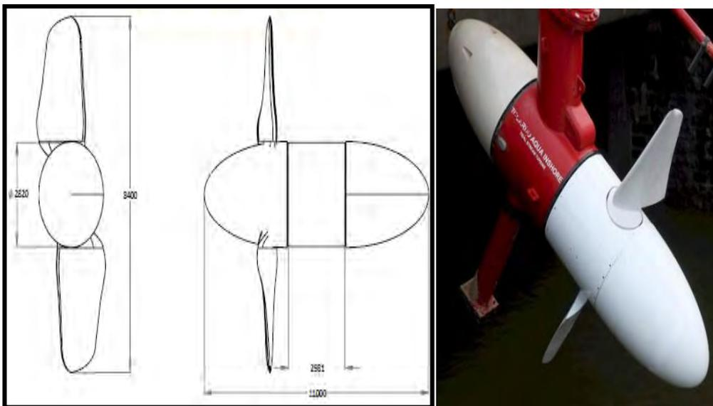
Figure 6.1.6.1: Design schematic of the Tocado T500-A Turbine (left) image of inshore Tocado turbine of same design(right) from Tocado International, 2012)
