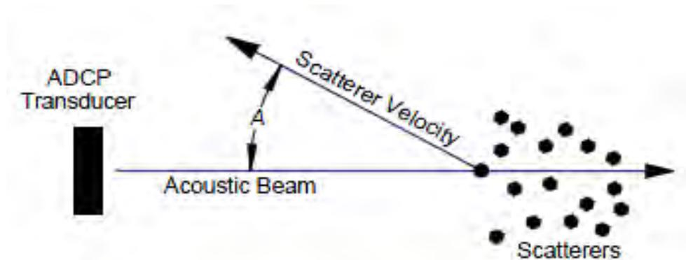
Figure 5.1.1: Relative velocity vector. The ADCP measures only the velocity component parallel to the acoustic beams. A is the angle between the beam and the water velocity (RD Instruments RDI , 1996).
