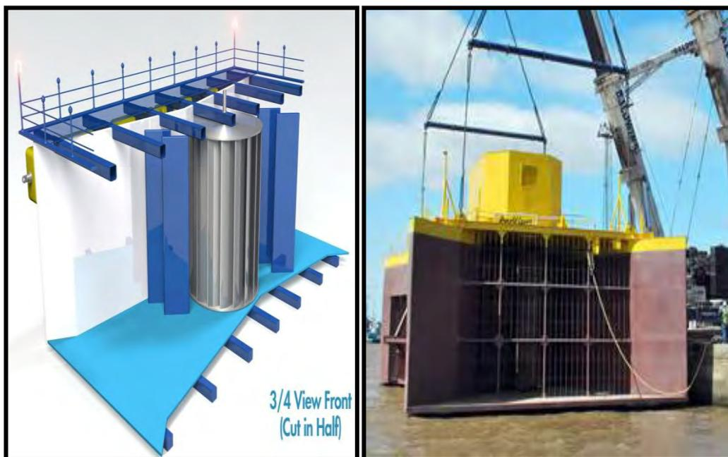
Figure 6.1.7.2: Simulation of Neptune Turbine  $\frac{3}{4}$  view front (left), side view of Neptune demonstrator being deployed (right) (NREL, 2012)
