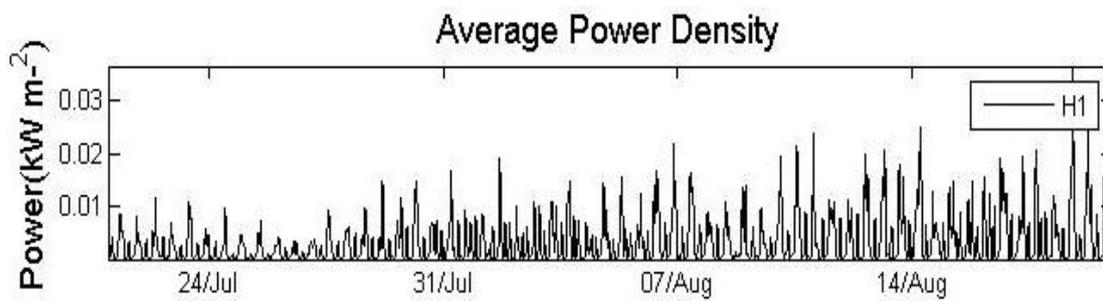
Figure 8.1.1.8: Average power density for long channel velocity component (V) at 5.3 meters from the bed, calculated over a 30 day period from the 21.07.11 to 20.08.11 for assessment site H1.
