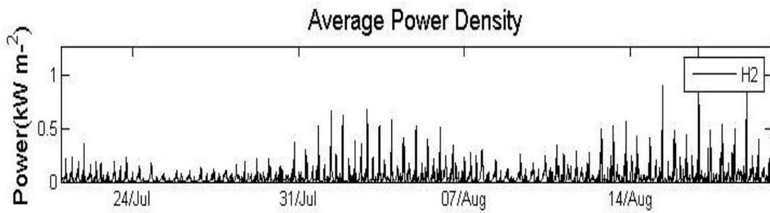
Figure 8.1.2.8: Average power density for long channel velocity component (V) at 9.9 meters from the bed, calculated over a 30 day period from the 21.07.11 to 20.08.11 for assessment site H2.
