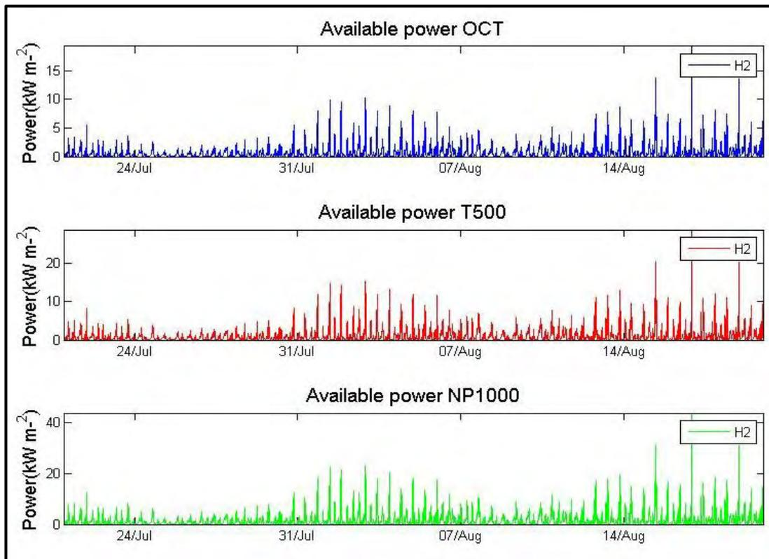
Figure 8.1.2.9: Extractable power output from OCT, T500 and NP1000 turbines assuming 100% power extraction independent of cut-in speeds for site H2 over one month.
