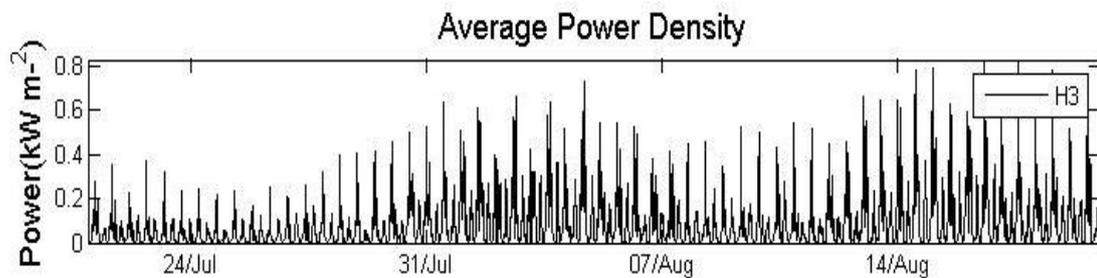
Figure 8.1.3.8: Average power density for long channel velocity component (V) at 5.9 meters from the bed, calculated over a 30 day period from the 21.07.11 to 20.08.11 for assessment site H3.
