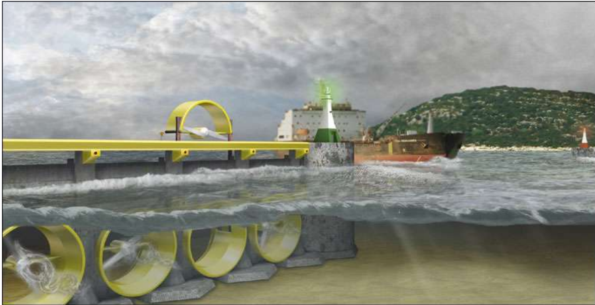
Figure 11: Conceptual tidal fence schematic 20
