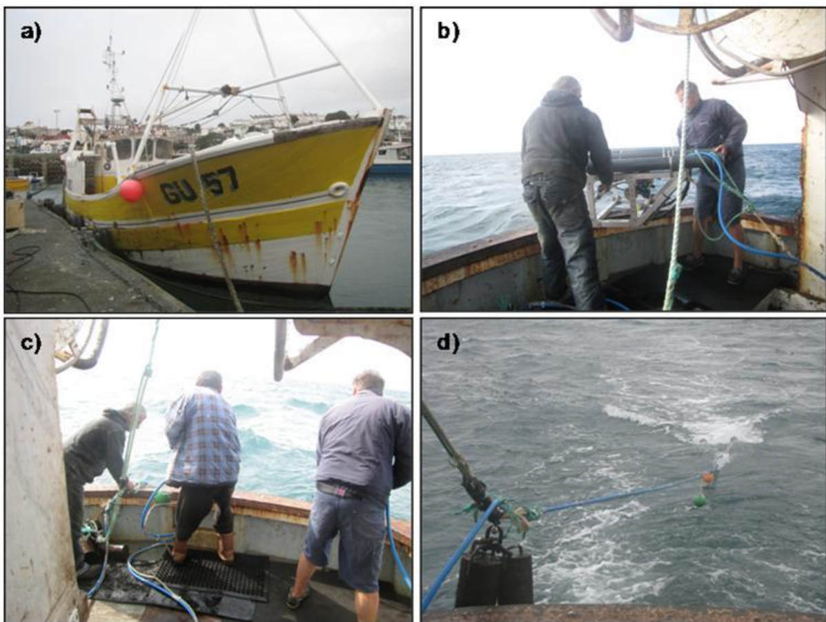
Figure 2.1: a) the vessel ‘Nicola May’ in port, b) & c) the flying array being deployed from the stern, d) the towed array emerging showing the umbilical (blue) and drop-weights for stability
