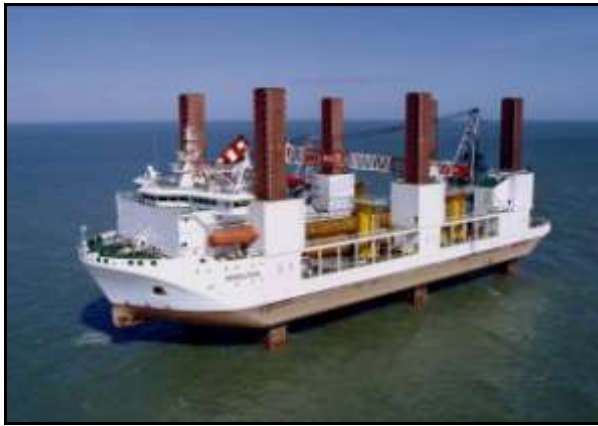
Figure 2.8 – MPI Resolution installation vessel about to install monopiles and transition pieces (photo - Courtesy of MPI)
