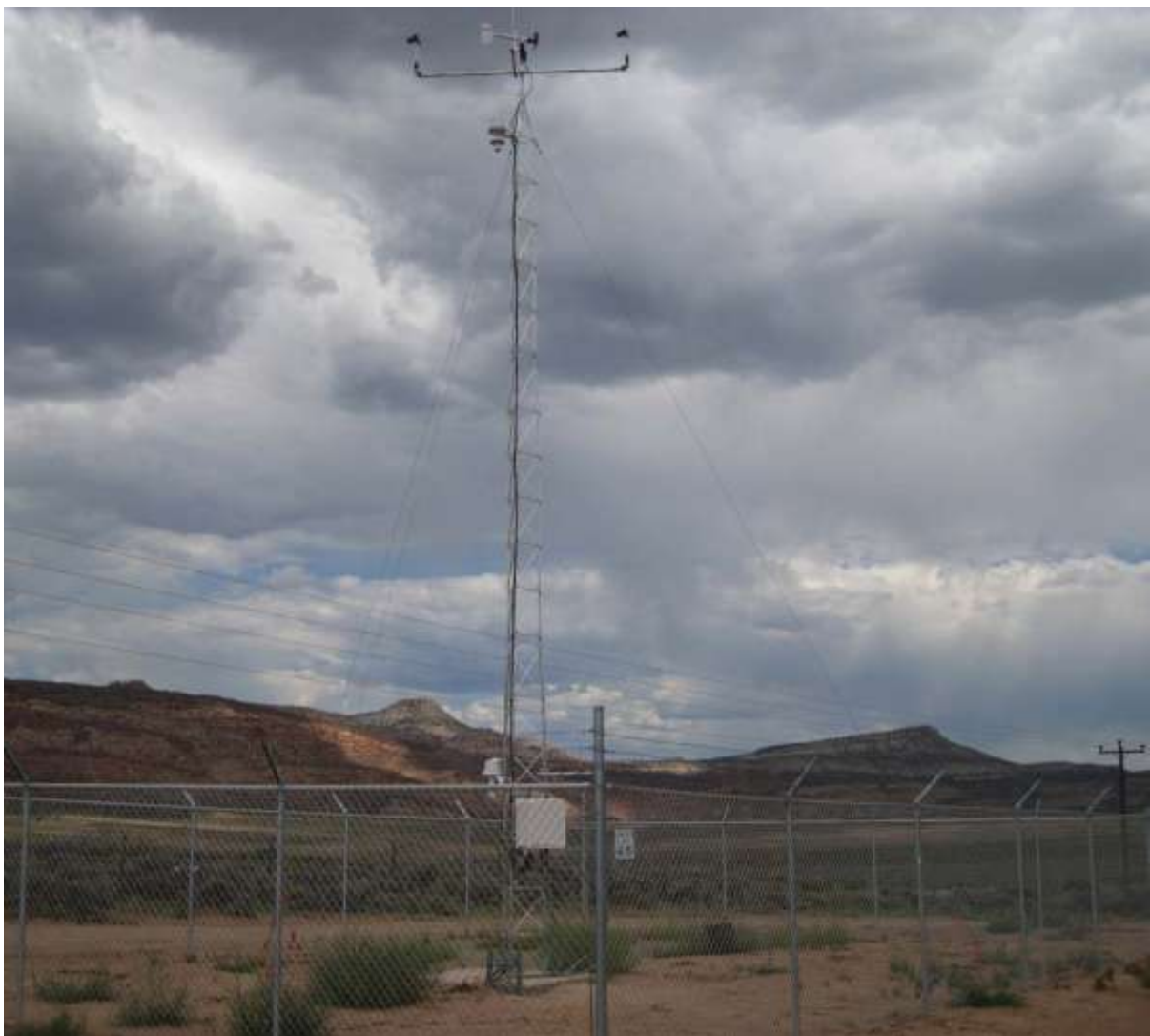
Fig.6 – Measuring wind direction & speed at 10 metres. Source: Campbell Scientific
